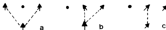
FIG. 4. Three instances of two successors: (a) nonneighboring successors; (b) successor directions differ by 60^\circ ; (c) successors in same direction.
