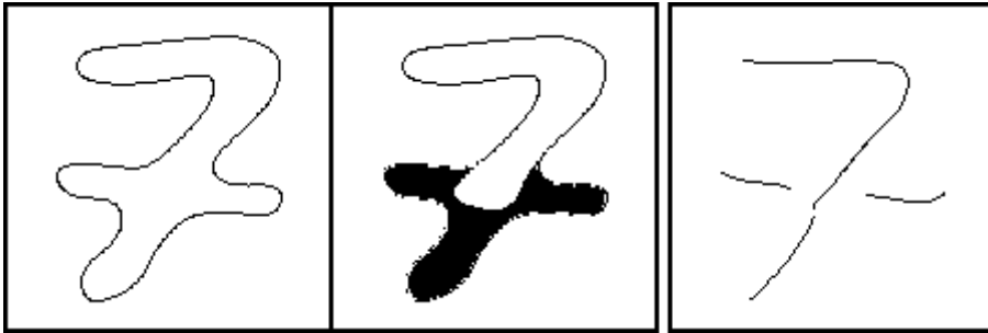
Figure 4.19: Decomposition and skeleton of a seven shape.
