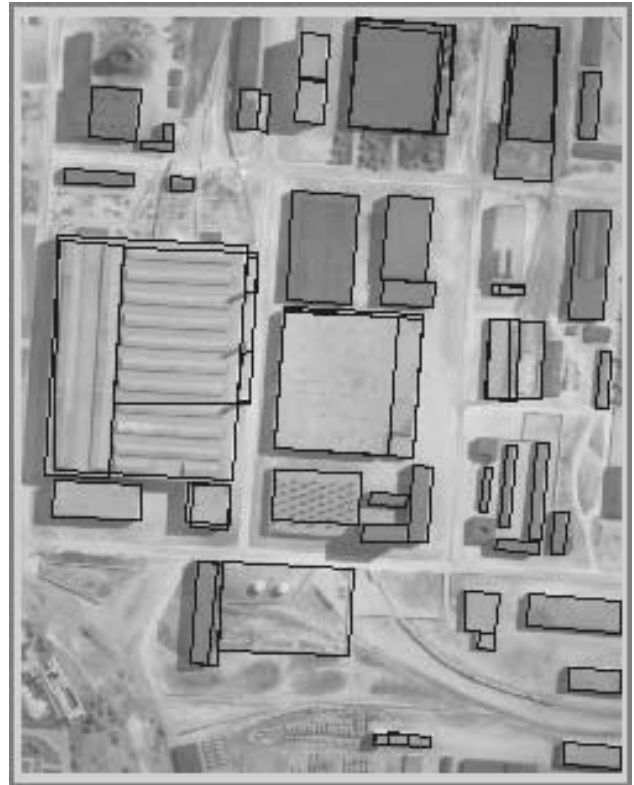
Figure 13 Automatically detected buildings from RADIUS modelboard image J3.
