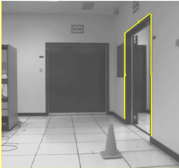
Figure 9 Indoor scene used for navigation with detected door outlined.
