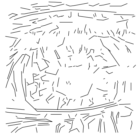
Figure 11: Extracted line segments from contours of length \geq 20 with e=5.0 , using a CM-5 partition of 32 PNs. Execution time \approx 347 msec
