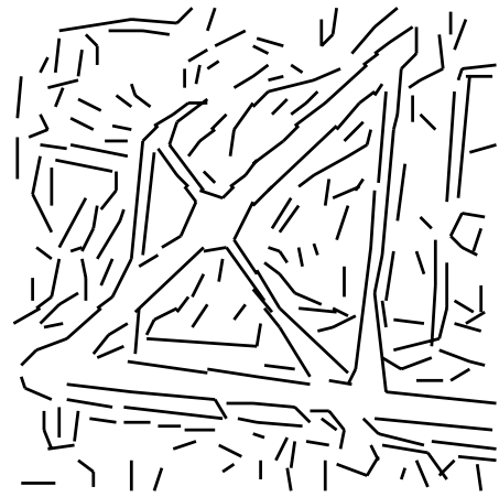
Figure 10: Extracted line segments from contours of length \geq 6 with e=3.0 , using a CM-5 partition of 32 PNs. Execution time \approx 96 msec
