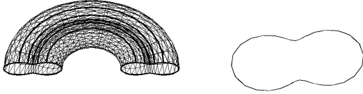
Figure 14: A PRCGC (left) and the recovered cross section (right). The top parabolic curves (and the terminations) are shown emphasized.
