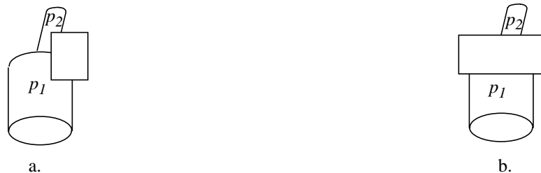
Figure 6.10 Joint detection allows for partial occlusion. a. a joint is marked between parts p_1 and p_2 .b. no joint is marked
