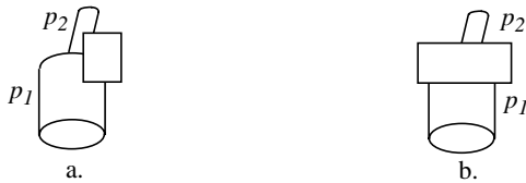
Figure 8 Joint detection allows for partial occlusion. a. a joint is marked between parts p_1 and p_2 ; b. no joint is marked
