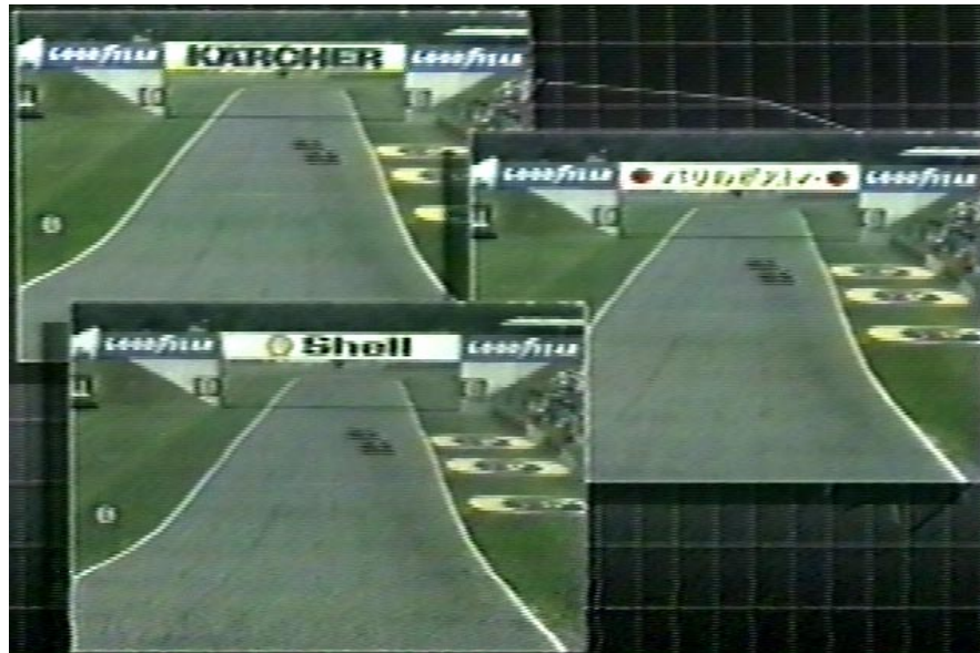
Fig. 1 The physical Shell billboard is replaced by virtual billboards, targeted for different audiences
