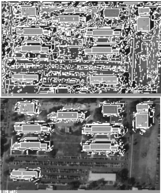
Figure 8. Linear segments in EO image (top) and those near IFSAR cues (bottom).
