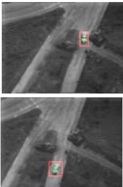
Figure 2: Tracking of a car going through a road block. The red rectangle corresponds to the bounding box of the moving object, and the green lines displays its motion direction.
