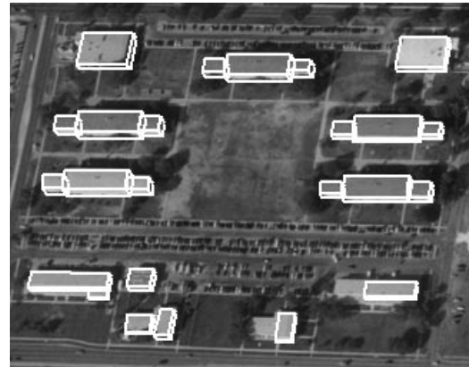
Figure 21 . Building components extracted using HYDICE cues.
