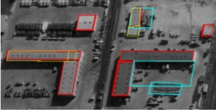
FIG. 8. Example hypotheses. Positive hypotheses are shown in red, negatives are blue, and the yellow ones are the don't care hypotheses.
