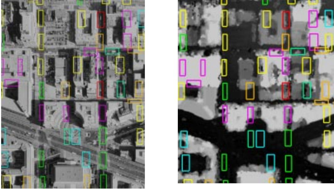
Figure 6 Before Using DEM for positioning. Road segments on image and on computed DEM. Green/Blue indicate relatively low elevation, red/purple relatively high.
