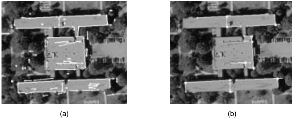
Figure 7. 2-D features which belong to the selected (a) 3-D linears; and (b) 3-D junctions. Polarities are shown with arrows.
