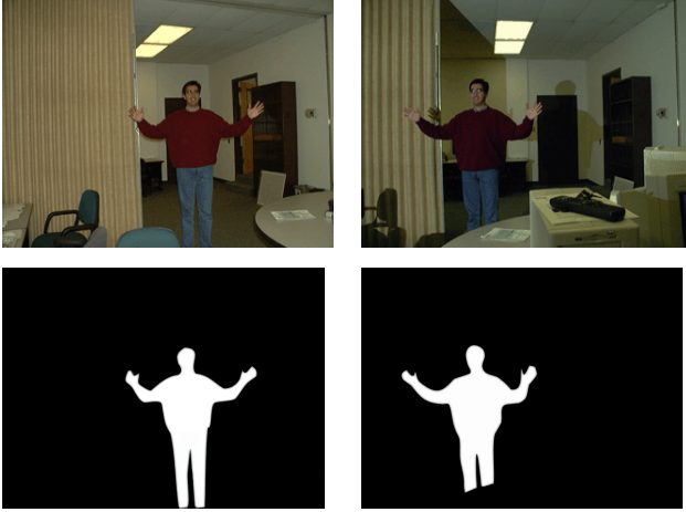
Figure 2: Body detection from a video stream. The two images correspond to two frames simultaneously acquired by two video cameras.
