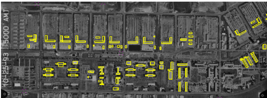
Figure 19 Model constructed from several sub-images using three views, displayed on a nadir image. This image is 7600x2700 pixels with GSD of 0.3 m, the oblique views have a smaller GSD (similar to other images of the same site shown elsewhere).
