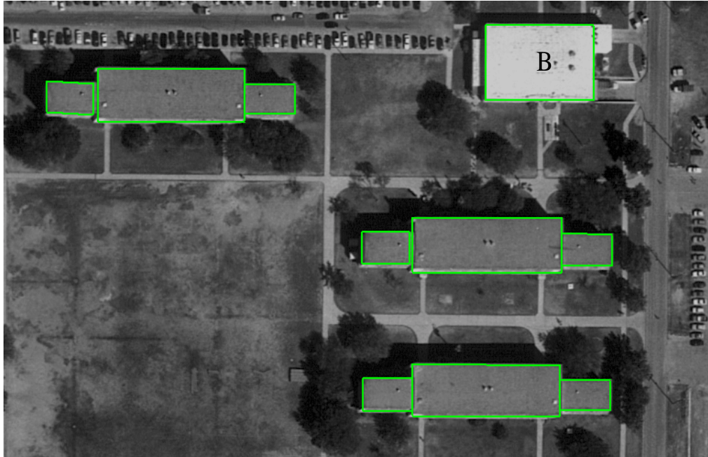
Figure 16 Gable-roof buildings detected as flat-roof buildings. Left image is 456x250 with GSD of 0.5m, right image is 450x215, GSD 0.4m
