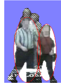
Figure 5: The likelihood based on the number of wrongly classified pixels. False positives: in white; true negatives: in shade. NOTE: single-ellipsoid model instead of 3-ellipsoid model is used for illustration.
