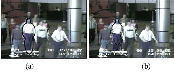
Figure 3: 3-ellipsoid human model. (a) The model is composed of 3 parts: head, torso and legs; (b) The 2D heights computed by camera model from a fixed head-top assuming the 3D heights are 1.6, 1.7 and 1.8 meters respectively.
