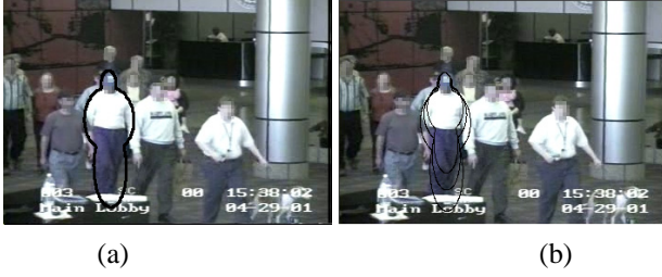
Figure 3: 3-ellipsoid human model. (a) The model is composed of 3 parts: head, torso and legs; (b) The 2D heights computed by camera model from a fixed head-top assuming the 3D heights are 1.6, 1.7 and 1.8 meters respectively.
