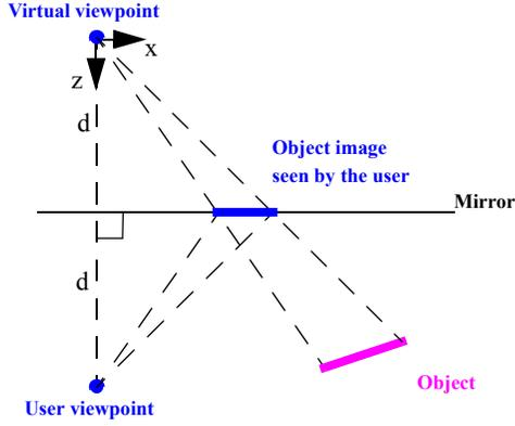
Figure 2. Mirror geometry.
