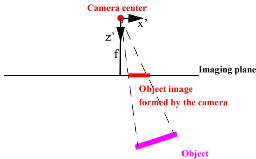
Figure 3. Pinhole camera geometry.
