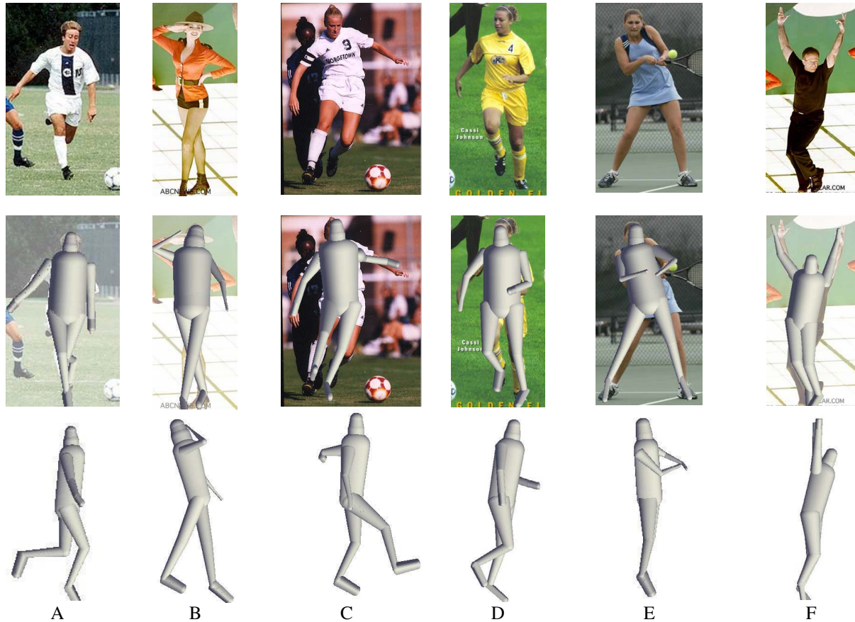
Figure 4: Pose Estimation. 1st Row: Original images, 2nd row: estimated poses, 3rd row: side view. Due to space limitation, the images were cropped for display. Errors include: (1) the person's left lower leg in image A, as it is mostly hidden, (2) the left arm in B, where the elbow is highly bent, (3) the left foot in C which is dark and similar to background, (4) the feet in E is wrongly estimated to be tip-toed. In addition, there are errors in depth estimates such as the right elbow in B, the tilting of the torso in B, the left feet in C, and the right arm in D.
