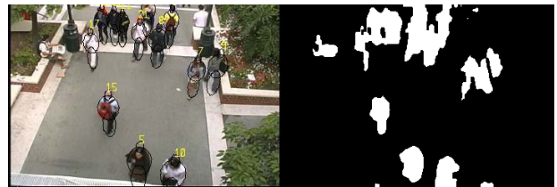
Figure 1: Left: a snap shot of our result overlaid on the input frame. Right: output of standard change detection shows the challenges to blob tracking and blob-based initialization.
