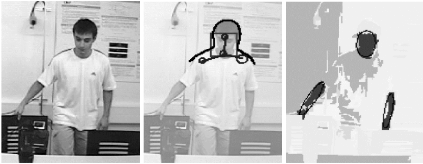
Fig. 2. Image observations, from left: (i) original image, (ii) detected face and head-shoulders contour, (iii) skin color ellipses extraction.
