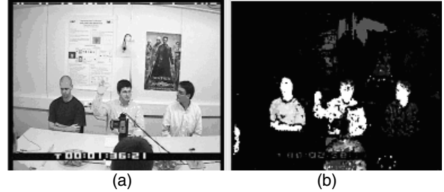
Figure 3: Target detection. (a) Original image. (b) Image intensity proportional to probability of the targets.
