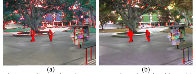
Figure 1. Comparison between two detection algorithms (a) Using a concatenation of affine transformation from the reference frame. (b) Using the proposed sliding window method
