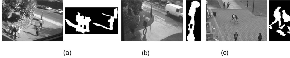
Fig. 1. Example moving blobs by change detection from three images in our dataset. One blob may contain multiple objects due to their proximity or camera projection (a), (c). It may also contain nonobject pixels such as shadow (sun shadow in (a) and soft shadow in (c)) or reflection (b). The foreground corresponding to an object may get fragmented (c).
