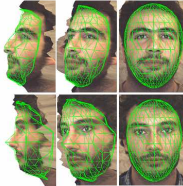
Fig. 6. Updated tracking meshes at different poses. The updated structure conforms well to the subject’s face.
