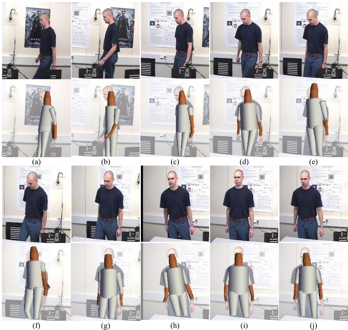
Figure 9. Dynamic pose estimation with PETS video with body turning movement. The person's right hand was occluded in (b) and (c), but its track was reestablished in (d) when it reappeared. There is also another period in (e) and (f) when the right hand was again occluded and the estimations were erroneous as the right hand was attracted to the skin regions around the left hand. Track was regained in (g).
