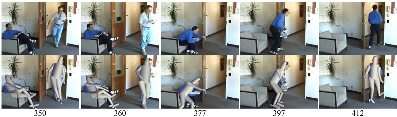
Figure 11. Tracking during video segment that includes two people and moving door. For the left person, errors include (i) the arms in Frame 360, 412, (ii) confusion of left and right arms in 377, and (iii) feet in 377, (iv) elbow in 397. For the right person, errors include (i) right foot in 350, (ii) left arm in 350, (iii) both arms in 360.
