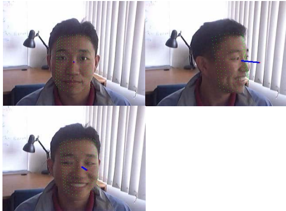
Figure 2: Results of 3D head pose estimation. The arrow indicates the direction and the green points are the points in the cylinder surface. The sequence starts from the upper left frame. The subject turns his head counterclockwise till near 45^\circ angle (the upper right image) and then turns back (the lower right image). When he moves his head, he makes a smile at the same time. These images show the 3D head pose estimation method has high accuracy even when there is an expression occurring along with the head movement.
