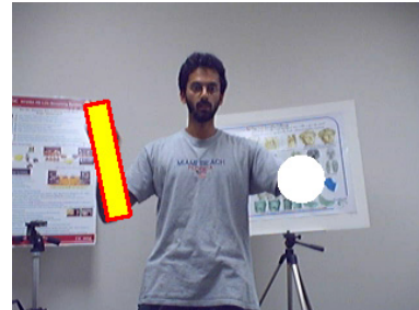
Figure 1: The output of our tracking system. Information such as the location of the arms as well as whether they point towards or away from the camera is useful in human-machine interaction.
