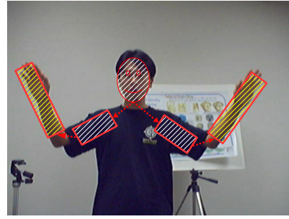
Figure 4: Articulated upper body model used for limb detection. The limbs are arranged in a tree structure as shown, with the head as the root. Between each parent/child pair their exists soft constraints. In our work we anchor the head at the location found from the people detection (section 3.2) module and only incorporate visual features of the forearm.
