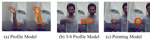
Figure 5: The tracking model represents an object as a collection of feature sites that correspond to either skin colored (at the intersection of the yellow lines) or a boundary pixel (red squares). The consistency of the model with the underlying image is measured as a weighted sum of the distance of the boundary pixels to the nearest edge pixel and the skin color scores under the skin feature sites.
