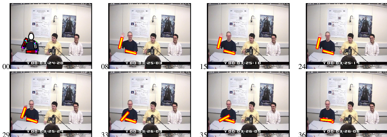
Figure 12: The results of the limb detector and tracker on a PETS sequence. In frame 0 the initial pose is detected and successfully tracked through frame 36.
