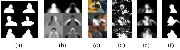
Figure 4. PCA based head-shoulder segmentation: a) training samples; b) eigenvectors. The left top one is the mean vector; c) original human samples; d) color probability map; e) PCA reconstruction; f) thresholded segmentation map.
