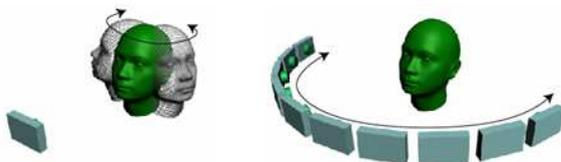
**Fig. 1.** The problem of reconstructing a single rigid object (static or mobile) with a single camera (static or mobile) can be equivalently modeled as reconstruction from multiple static cameras with the same relative external coordinate system
