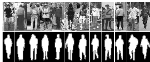
Figure 4. Samples for frontal/rear view pedestrian: the first row is the image samples; the second row is the segmentation ground-truth (The grey pixels are do-not-care).
