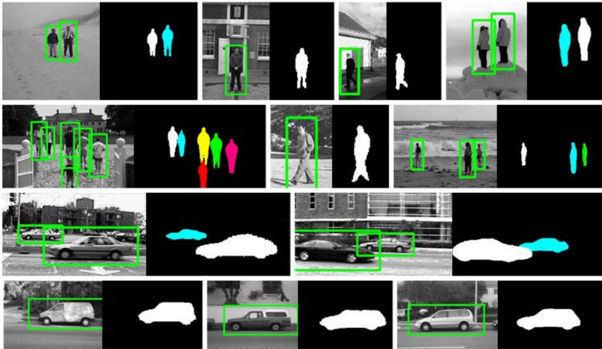
Figure 10. Examples of detection and segmentation results: for each pair left is the detection result and right is the segmentation result. When there are multiple objects, different colors represent different objects. When there are overlap between two objects, we assume the object with larger y -coordinate (assume the left-top corner of the image is (0,0) ) is closer to the camera.
