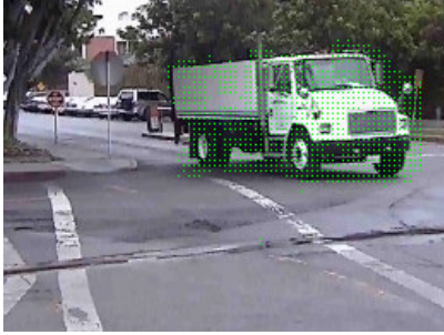
Figure 4. The raw segmentation by Tensor Voting in truck sequence; green dots are the obtained result after outlier refinement step.
