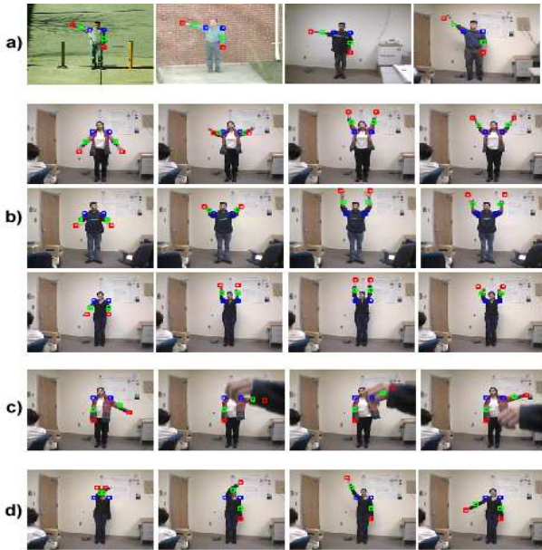
Figure 6. Recognizing and tracking with variation in - a)Background and Lighting b) Style c) Random external motion d) Self-Occlusion
