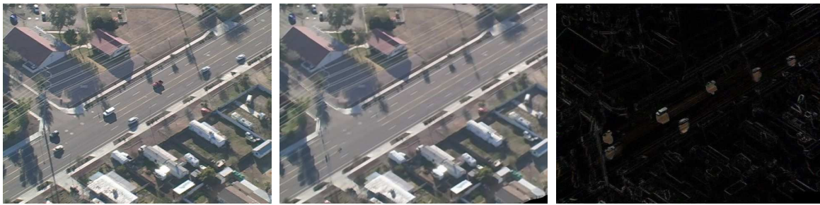
(a) Reference frame (b) Background model at the reference frame (c) Motion mask at the reference frame
