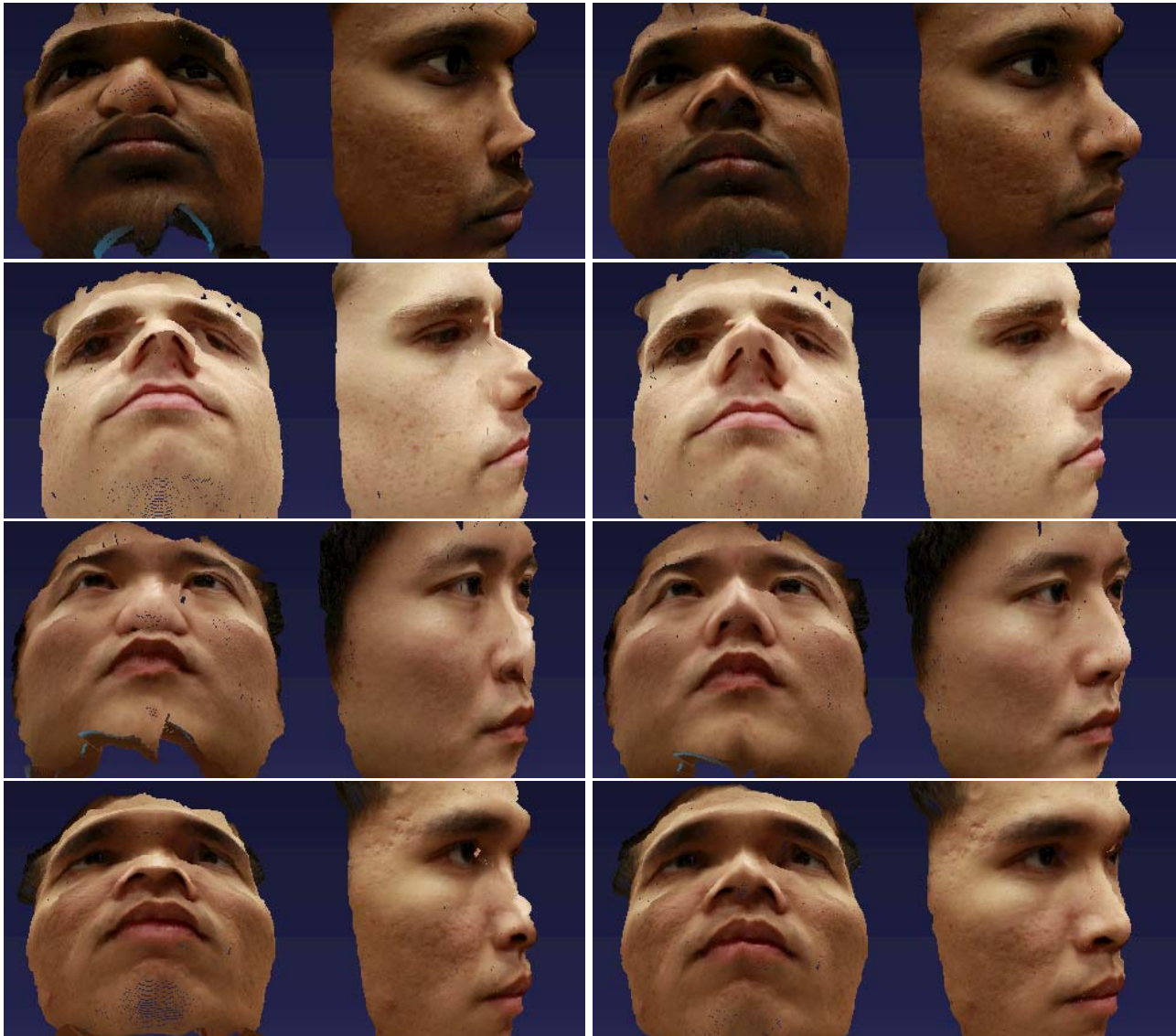
Figure 9. Reconstruction of real images (291600 points rendered in MeshLab [5]): without profile contours (left) vs. with profile contours (right).
