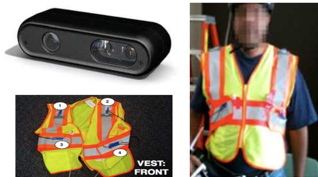
Fig. 1. A RGB-D camera on the top left and a tactile vest interface device on the bottom left. RGB-D camera operates with USB interface and tactile interface system communicates via Zigbee wireless network
