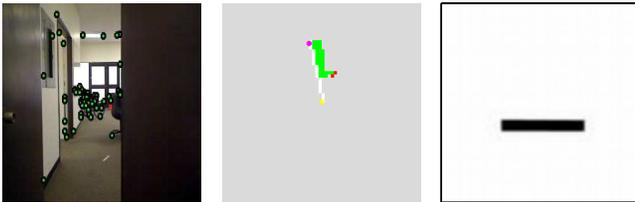
Fig. 6. Visual odometry and SLAM result. Left: RGB-D camera image with feature points extracted. Center: Traversability map with path finding algorithm. White bar show the safe path to the way point. Right: Calculated cue based on traversability map (Go straight).
