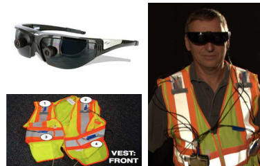
Figure 1. The wearable navigation system consists of a stereo camera with a vest-type feedback system.
