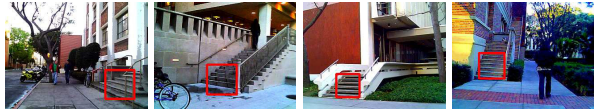
Figure 3. Staircases detected using the proposed algorithm are shown. Note that the proposed algorithm can detect staircases from various view points and lighting conditions
