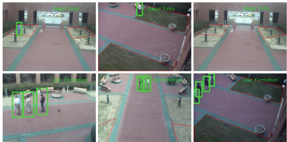
Fig. 7 Event detection results (illegal entry event detection (top row), line formation event detection (bottom row))
