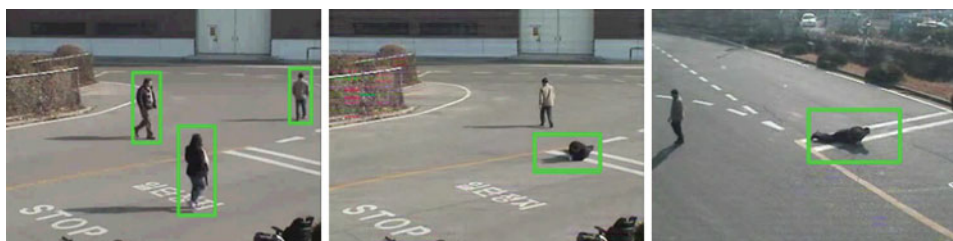
Fig. 6 Examples of human detection in different poses ( left: standing and walking, middle and right: lying down )
