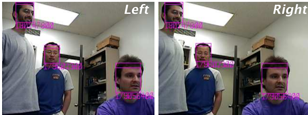
Figure 1: Composite images of tracking data overlaid on left and right input color images. Note the head area size consistent with the person’s distance to the cameras (the further away, the smaller) and the consistent labels in the left and right views.
